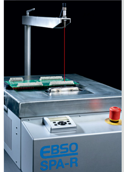
SPA-R with laserpointer to ease component centering over nozzle
