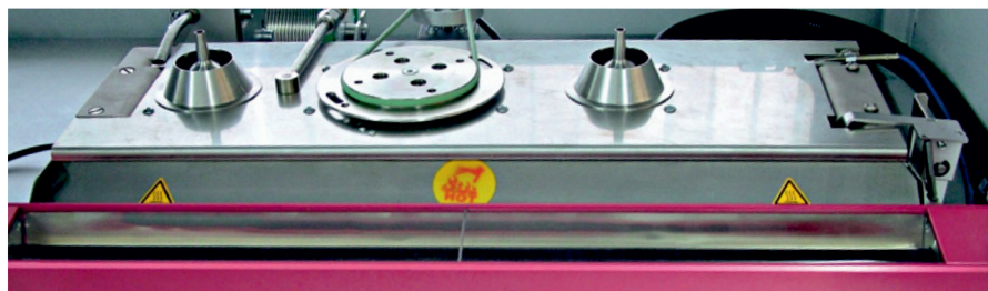
Solder pot with dual nozzle technology and IR-preheat
