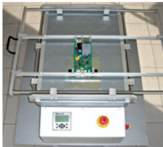
XY-Table with position fixing
