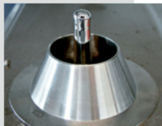
Miniwave with overflow wettable solder nozzle
