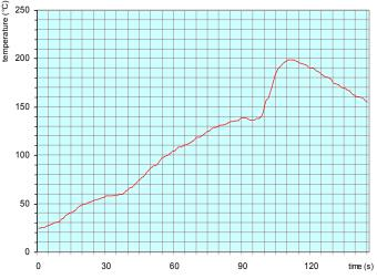
To measured on the topside of the PCB on a lead-free wave soldering machine.
