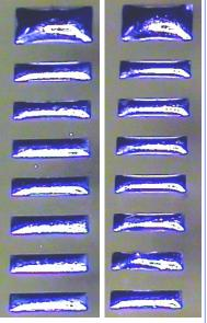
Left: micro solder balls with conventional VOC-free flux Right: 2009MLF
